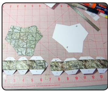
For the larger, stand-alone elevations, the construction process is slightly different. Cut and score the pieces as shown.
